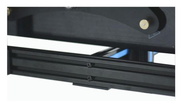
Step 5. Tighten the screws on the  $\boldsymbol{Z}$  axis stators.
