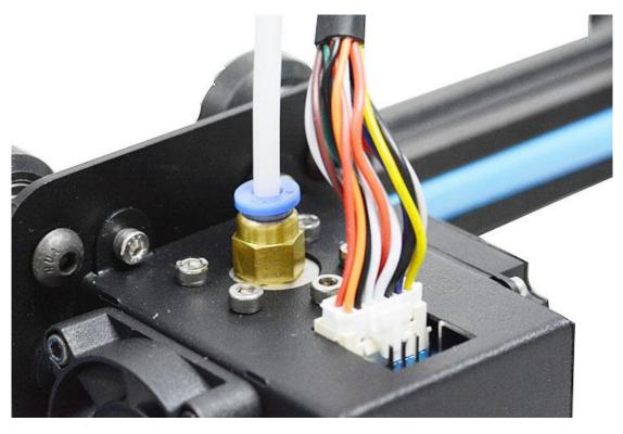
Step 7. Attach the filament holder kit to the control box with 2 \* M3\*6mm.
